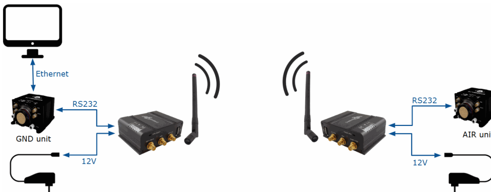
Microhard radios and Autopilot 1x operation
